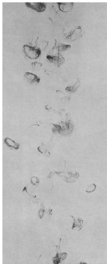
Fig. 5. The vortex rings formed behind the drop in a Class VI wake are in evidence. Reynolds number 1010.
